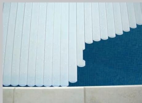
4. Hand processing of roman ends and cut-outs. Final cleaning and inspection.
