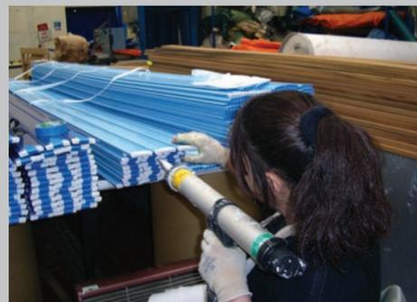
3. End caps being siliconed using pneumatic pressure silicone guns.
